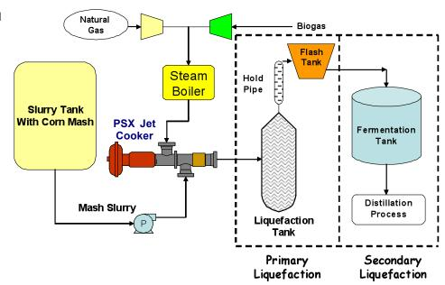
In the Primary Liquefaction Stage, slurry is then pumped through a pressurized jet cooker at 221°F and held for 5 minutes. The mixture is then cooled by an atmospheric or vacuum flash condenser. After the flash condensation cooling, the mixture is held for 1–2 hours at 180–190°F to allow the enzymes time to work.
