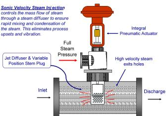
control valve or downstream mechanical mixing devices. *High velocity steam flow* optimizes the steam mixing and condensation with the liquid and eliminates problems with vibration/steam hammer.
