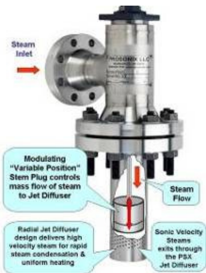
PSX Jet Diffuser Internal View
