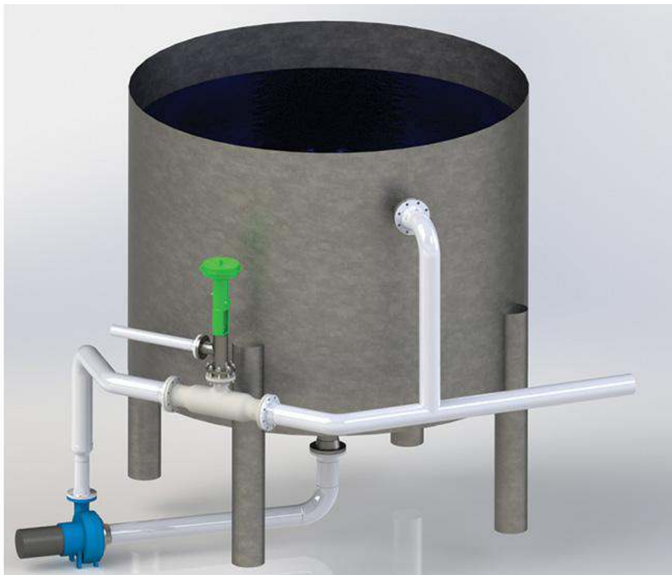
FIGURE 3. Hot water tank recovery after drawdown can be slow and may affect the availability of hot water. Using an external inline steam-injection heater may provide better performance.
