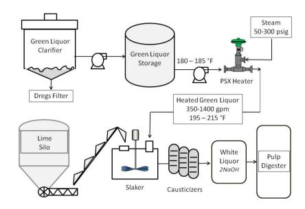
Kraft Pulp mills produce pulp from wood chips. Within the pulp production, a chemical process produces green liquor. Green liquor is a combination of recovery boiler smelt, and dilute white liquor. Dregs are removed and liquor is sent to recausticizing tanks to produce white liquor. Flows vary based on the size of the pulp mill and can range from 350-1400 gpm.
